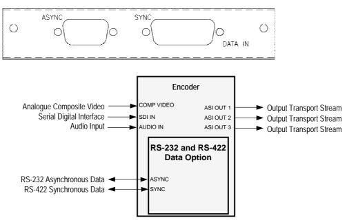
Figure 3.2: RS-232 and RS-422 Data Input Option M2/EOM2/DAT
